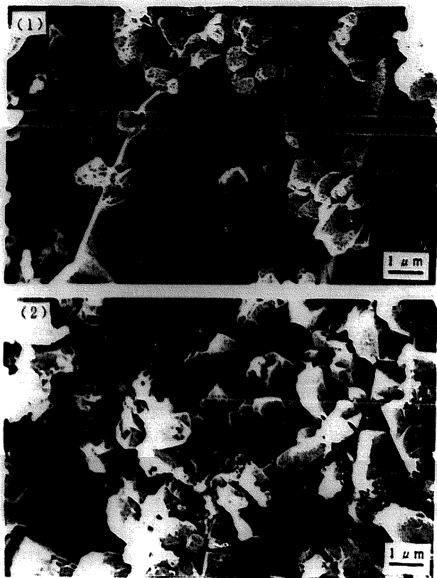
Fig. 10. SEM micrographs of the positive electrodes: (1) after charging with CC (0.2 C)–CC (0.05 C) for 224 cycles, (2) after charging with CC (0.5 C)–CC (0.05 C) for 280 cycles.
